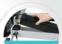
Battery pack removes wit anti-theft key for easily trading to a fresh battery.
