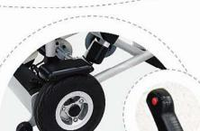
Standard safety features include a loud beeper horn and anti-tip rear wheels.
