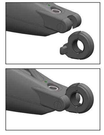
1. To attach the drive unit to the wheelchair, align the flats in the adaptive clamp with the receiving slots on the front, underside of the unit body [the drive unit will be angled slightly higher than horizontal]. Lower the receiving end of the drive unit over the extrusions of the clamp.
