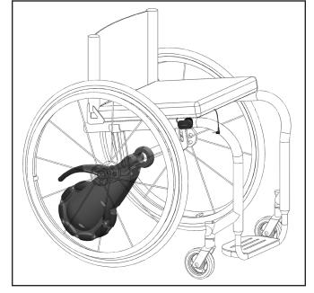
**3.** Under its own weight, the omni-wheel end of the drive unit rests on the ground between the rear wheels of the wheelchair.
