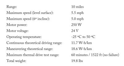
NOTE: The stated values are from testing with a 250 lb. occupant. The range, speed, etc. vary depending on driving conditions.
