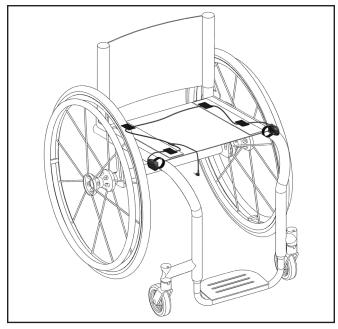
2. Use the provided velcro strips to strap down the button cables to the upholstery, running the right button cable around the back of the seat. Ideal placement of the y-joint in the cable is shown to the right. Be be sure the cable does not stick out and will not get caught in the spokes of the wheelchair.
