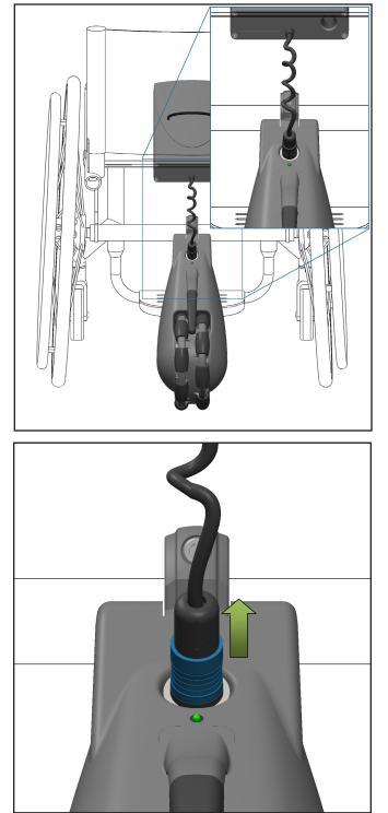
5. To unlock and disconnect the battery from the drive unit, pull up on the outer sleeve of the connector (highlighted in blue in the figure to the right).
