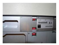
The red plugs are electrical contacts between the Braille display and the module. The ribbon-cable supplied with the module is inserted into this connector. Finally, the facing can then be screwed onto the module.
