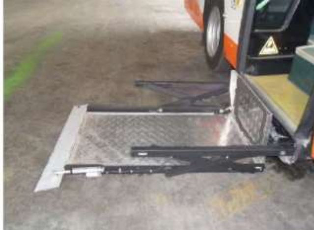
Figure 115- Platform installed under step of bus
